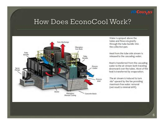
The EconoCooler is a custom engineered field-erected industrial heat exchanger engineered, designed, and guaranteed by J. D. Cousins.
